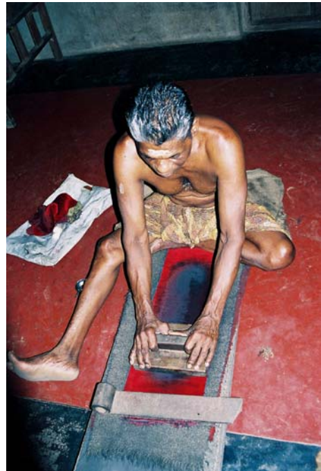
Mirrors: Metal Mirrors from India. Fig. 5 Polishing of cast blank on hessian cloth using the powdered brittle mirror alloy itself for polishing.
